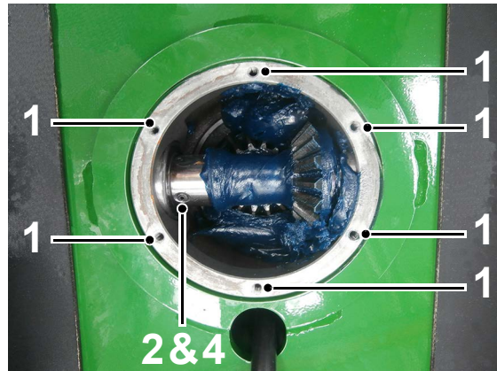
Gearbox cross shaft pin replacement
